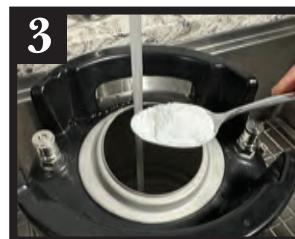
Remove the pour spout assembly and fill the keg with hot water and 1 Tablespoon of baking soda.
