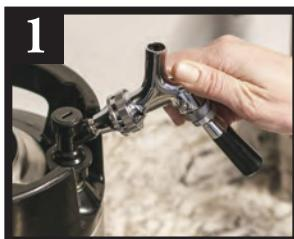
With the pour spout assembly attached to the keg, pull the lever forward to open the tap and rotate 180°. This partially unscrews the spout from the ball lock.
