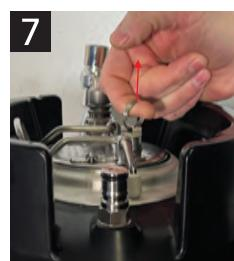
7. The pressure is increased by turning the dial clockwise and released by pulling on the pressure release valve ring. Set the pressure to 5-7 psi. Mixing or traveling can increase the pressure so be sure to check the gauge before use.
