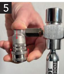
5. To attach the regulator, first use fingers and thumb to retract the metal connection ring of the ball lock. *Note - Periodically spray the inside of the ball lock with non-stick cooking spray to protect the rubber seal in the keg post.*
