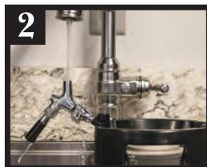
Run hot water through the spout and down through the pick-up tube. Reach your hand inside and wipe any residue.
