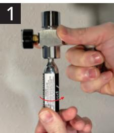
1. Ensure the regulator is off by turning the dial counterclockwise. Attach a CO<sub>2</sub> cartridge by completely threading it onto the regulator clockwise quickly and firmly.
