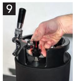
9. Attach the pour spout assembly to the keg by retracting the plastic connector with fingers and thumb. Then firmly press straight down onto the “OUT” Post of the keg. Release the connector and make sure it is fully seated.
