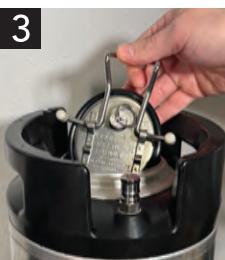
3. Attach the lid. Place the longer side of the lid into the keg, then rotate it 90° to align it with the keg opening.
