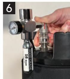
6. Attach the regulator to the keg by firmly pressing the retracted connector straight down onto the “IN” post of the keg. Release the connector and make sure it’s fully seated.
